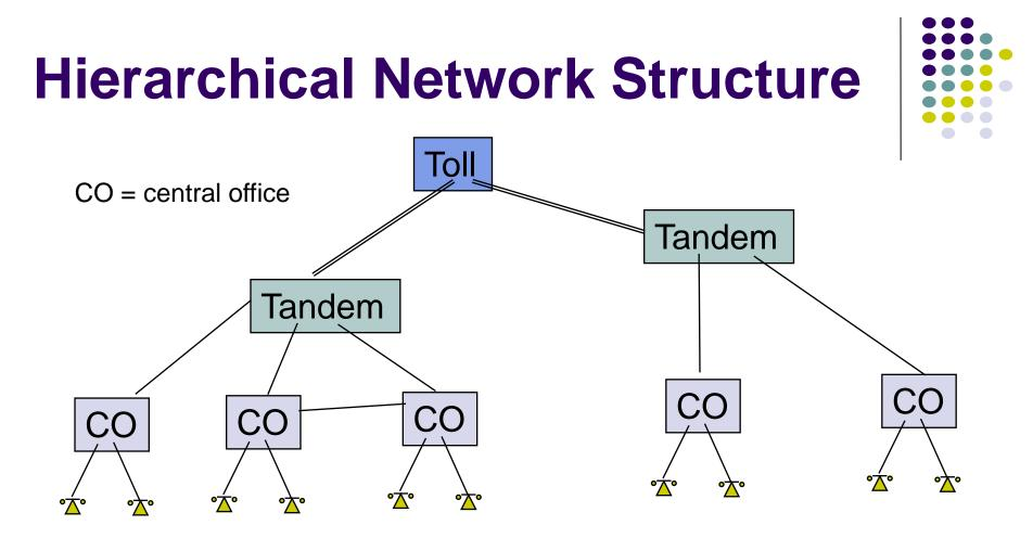
Telephone subscribers connected to local CO (central office) Tandem & Toll switches connect CO's
