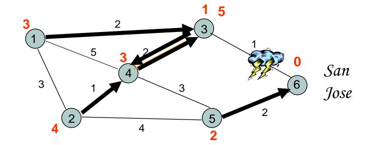
Network disconnected; Loop graded between nodes 3 and 4
