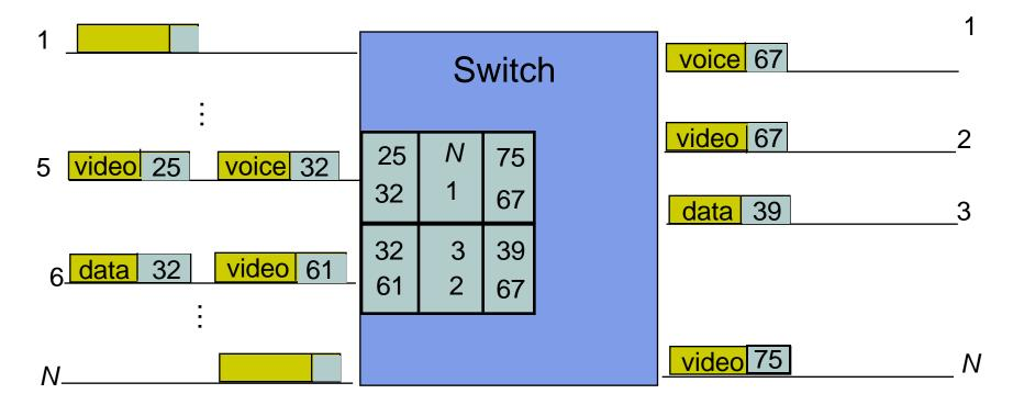
ATM switches can be implemented using shared memory, shared backplanes, or self-routing multi-stage fabrics
