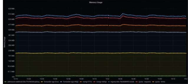
Fig. 10: NSM control plane components memory size usage during SFC deployment
