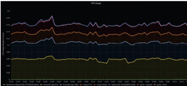
Fig. 9: NSM control plane components CPU unit usage during SFC deployment
